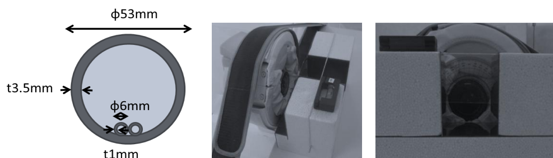
Figure 1: A phantom in MRI device. The phantom size (left). The phantom was stabilized horizontally referred by a level meter (middle). The rotation angle of the phantom in static MR imaging was set according to a goniometer (right).
